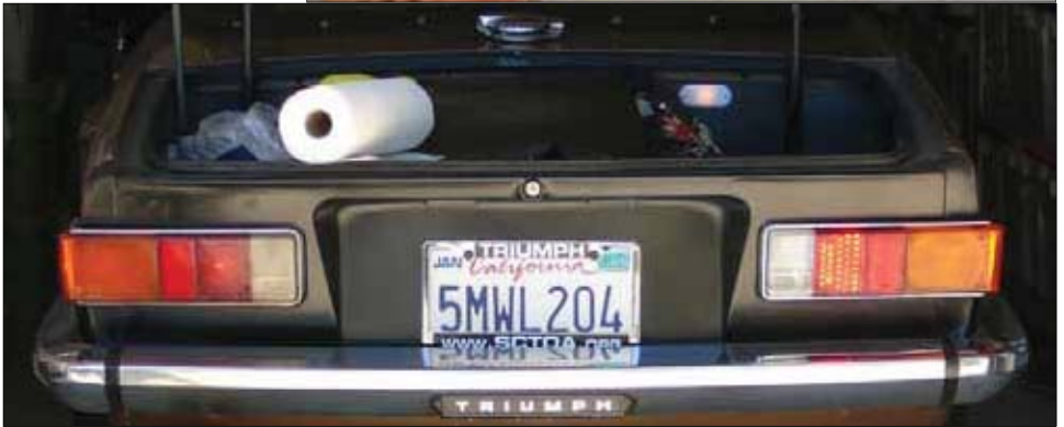
Lights ON - original light bulb is still in the left; new LEDs are in the right.
