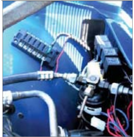
Added fuse block
